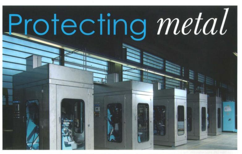
The modules of Sprimag's HIL-15 coating machine can handle 900 cans per minute each
