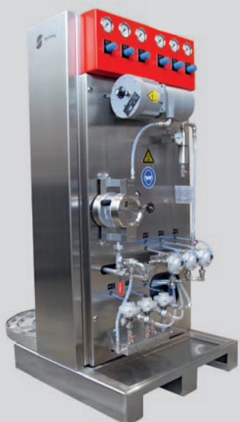
The different control circuits enable changing the layer thickness at the can bottom independently of the layer thickness at the can wall.
