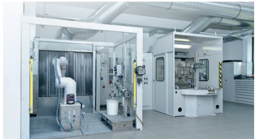
A compact robot stand and a special automatic round-table coating machine round off the range of services in the Applications Center
