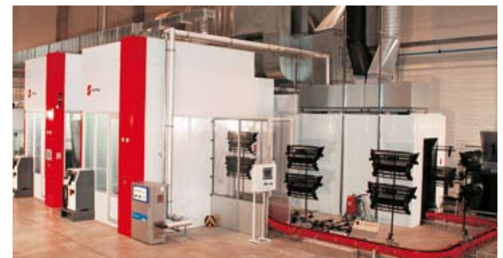
The new machine is coating radiator grills for AUDI.
