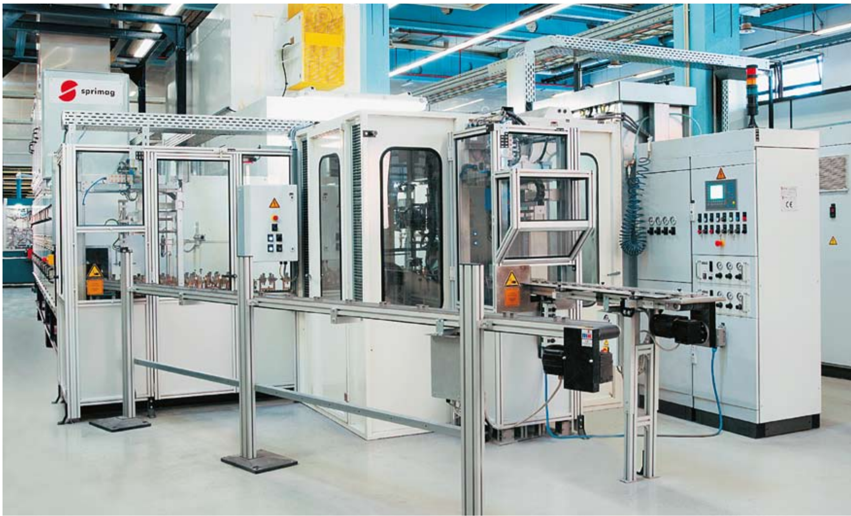
Connector housings of different sizes may be powder coated with this machine.
