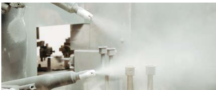
Top left: Hans Peter Dähn, Industrial Engineer HARTING, is convinced by the Sprimag technology. Top right: The infrared drier is responsible for a quick coagulation of the powder. Below: Powder station inside the Round Table Coating Machine.
