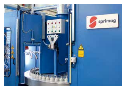
On the compact Round Table Machine engine components are automatically coated with anti-friction paint
