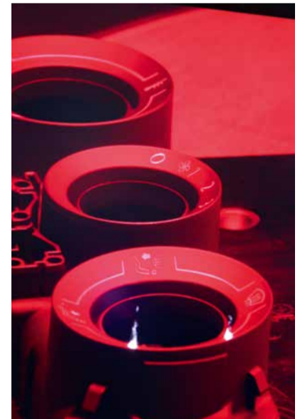
The first customer of Sprimag Brasil had an interest in lasered day and night-plastic parts.
