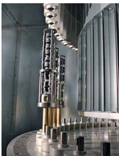
Dryer with air nozzles for uniform drying of the internal coating
