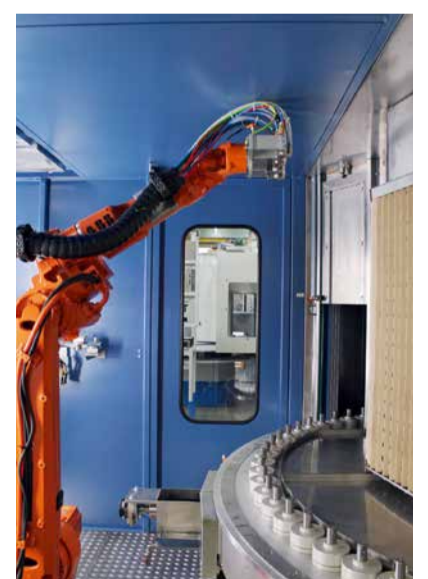
Thanks to the quick-release system readjustment of the spray guns is unnecessary
